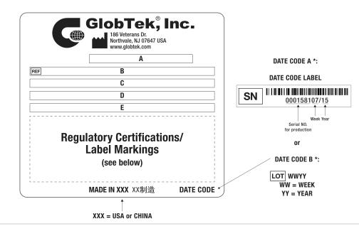
A=ICT / ITE / Medical Power Supply/Class 2/Household Power Supply B=P/N: (料号) RR9KE5000LCPCIMR6B C=Model (型号) GTM96600-6012-R2 D=Input (输入)100-240V~, 50-60 Hz, 1.5 A E=Output (输出)12.0 V === 5.0 A, 60.00W
