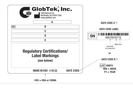
A=ICT / ITE / Medical Power Supply/Class 2/Household Power Supply B=P/N: (料号) RR9KA4500T00NAIMR6B C=Model (型号) GTM96300-2307.5-2.5-R2 D=Input (输入)100-240V~, 50-60 Hz, 1A E=Output (输出)5.0 V ---- 4.5 A, 22.50W
