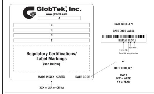
A=ICT / ITE / Medical Power Supply/Class 2/Household Power Supply B=P/N: (料号) RR9KA4500T00-IMR6B C=Model (型号) GTM96300-2307.5-2.5-R2 D=Input (输入)100-240V~, 50-60 Hz, 1A E=Output (输出)5.0 V ---- 4.5 A, 23.00W
