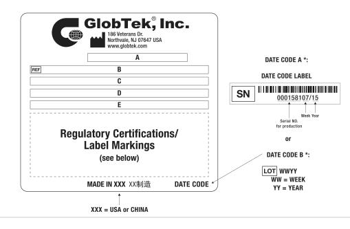
A=ICT / ITE / Medical Power Supply/Class 2/Household Power Supply B=P/N: (料号) RR9KA4500CCP-IMR6B C=Model (型号) GTM96300-2307.5-2.5-R2 D=Input (输入)100-240V~, 50-60 Hz, 1A E=Output (输出)5.0 V ---- 4.5 A, 22.50W
