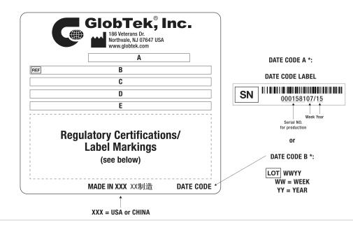
A=ICT / ITE / Medical Power Supply/Class 2/Household Power Supply B=P/N: (料号) PR9SY1800A00-IMR6B C=Model (型号) GTM96600-6536-P2 D=Input (输入)100-240V~, 50-60Hz, 1.5A E=Output (输出)36.0 V ---- 1.80 A, 65.00W
