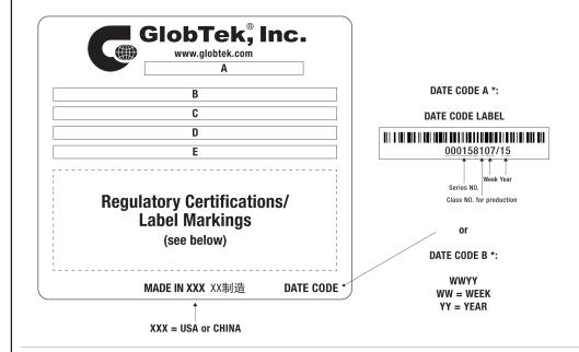
A=ICT / ITE / Medical Power Supply/Class 2/Household Power Supply B=P/N: (料号) PR9SA8000A00-IMR6B C=Model (型号) GTM96600-4005-P2 D=Input (输入)100-240V~, 50-60Hz, 1.5A E=Output (输出)5.0 V == 8.0 A, 40.00W
