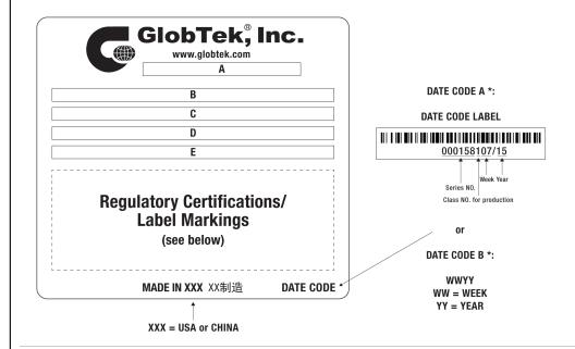
A=ICT / ITE / Medical Power Supply/Class 2/Household Power Supply B=P/N: (料号) PR9QI833KC2CHM(RVB C=Model (型号) GTM93021-2024-P2 D=Input (输入)100-240V~, 50-60 Hz, 0.6A Max E=Output (输出)24.0 V === 0.833 A, 20.00W
