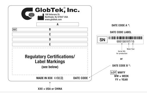
A=ICT / ITE / Medical Power Supply/Class 2/Household Power Supply B=P/N: (料号) PR91Z3250T00-IMR6B C=Model (型号) GTM96600-6520-P2 D=Input (输入)100-240V~, 50-60Hz, 1.5A E=Output (输出)20.0 V === 3.25 A, 65.00W
