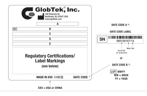
A=ICT / ITE / Medical Power Supply/Class 2/Household Power Supply B=P/N: (料号) PR91I2700T00-IMR6B C=Model (型号) GTM96600-6524-P2 D=Input (输入)100-240V~, 50-60 Hz, 1.5A E=Output (输出)24.0 V === 2.7 A, 65.00W
