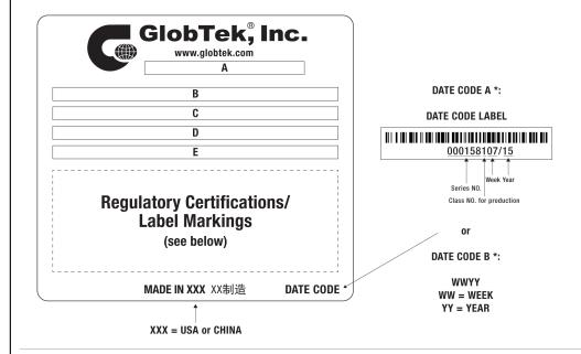
A=ICT / ITE / Medical Power Supply/Class 2/Household Power Supply B=P/N: (料号) PR91G4333CCP-IMR6B C=Model (型号) GTM96600-6515-P2 D=Input (输入)100-240V~, 50-60 Hz, 1.5A E=Output (输出)15.0 V == 4.33 A, 65.00W
