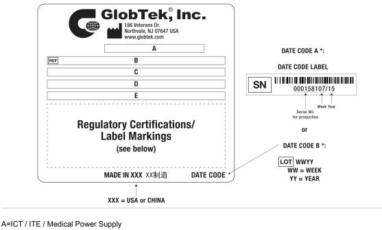
B=P/N: (料号) GTM962252P22512-FW C=Model (型号) GTM962252P22512-FW D=Input (输入)100-240V~, 50-60 Hz, 3A E=Output (输出)12.0 V === 18.75 A, 225.00W
