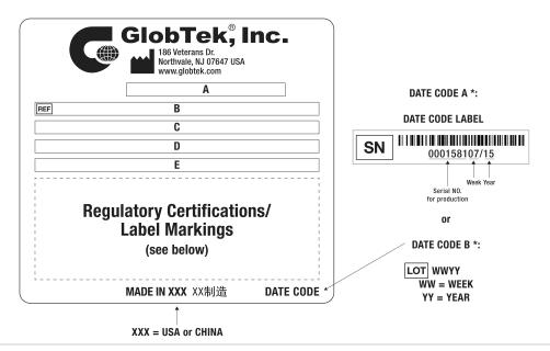
A=ICT / ITE / Medical Power Supply B=P/N: (料号) GTM962251P22554-FW C=Model (型号) GTM962251P22554-FW D=Input (输入)100-240V~, 50-60 Hz, 3A
