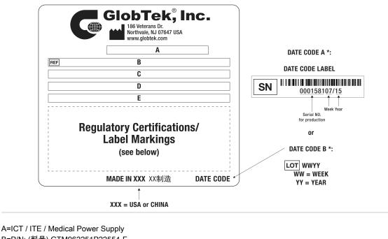
B=P/N: (料号) GTM962251P22554-F C=Model (型号) GTM962251P22554-F D=Input (输入)100-240V~, 50-60 Hz, 3A E=Output (输出)54.0 V === 4.16 A, 225.00W
