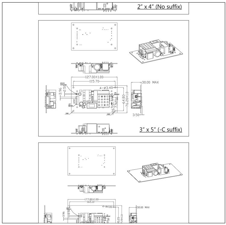
Drawing Title: GTM962250P22554A-F, ICT / ITE / Medical Power Supply, Efficiency Level: USA DOE Level VI / Eco-design Directive 2009/125/EC, (EU) 2019/1782, Case Color/Style: GlobTek Black, Open Frame/ L Frame/Cage/ Potted Internal, Regulated Switchmode AC-DC Power Supply AC Adaptor, Input Rating: 100-240V~, 50-60 Hz, PCB Pins, , Output Rating: 225.00W, 54.0V@4.16A, Pin Out: Pins 1, 2, 3: DC COM Pins 4, 5, 6: +V, Approvals:
