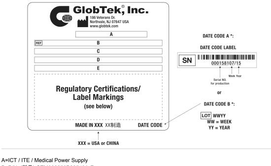
B=P/N: (料号) GTM962250P22548A-F C=Model (型号) GTM962250P22548A-F D=Input (输入)100-240V~, 50-60 Hz, 3A E=Output (输出)48.0 V === 4.68 A, 225.00 W
