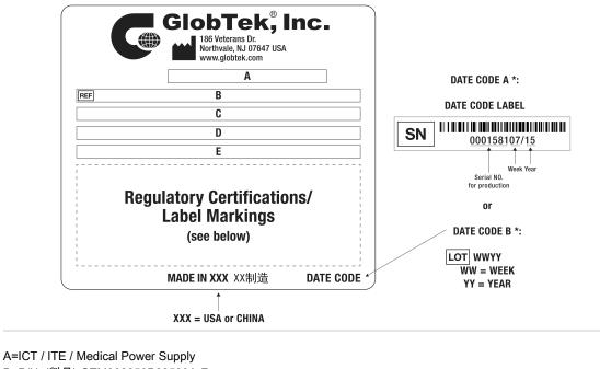
B=P/N: (料号) GTM962250P22530A-F C=Model (型号) GTM962250P22530A-F D=Input (输入)100-240V~, 50-60 Hz, 3A E=Output (输出)30.0 V === 7.5 A, 225.00 W
