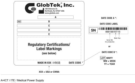
B=P/N: (料号) GTM962250P22528A-F C=Model (型号) GTM962250P22528A-F D=Input (输入)100-240V~, 50-60 Hz, 3A E=Output (输出)28.0 V === 8.03 A, 225.00 W
