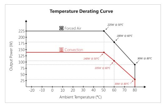
Drawing Title: GTM962250P22520A-F, ICT / ITE / Medical Power Supply, Efficiency Level: USA DOE Level VI / Eco-design Directive 2009/125/EC, (EU) 2019/1782, Case Color/Style: GlobTek Black, Open Frame/L Frame/Cage/ Potted Internal, Regulated Switchmode AC-DC Power Supply AC Adaptor, Input Rating: 100-240V~, 50-60 Hz, PCB Pins, , Output Rating: 225.00W, 20.0V@11.25A, Pin Out: Pins 1, 2, 3: DC COM Pins 4, 5, 6: +V, Approvals:
