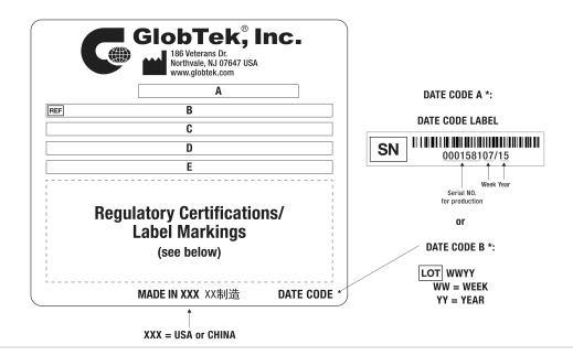
A=ICT / ITE / Medical Power Supply B=P/N: (料号) GTM962250P22518A-F C=Model (型号) GTM962250P22518A-F D=Input (输入)100-240V~, 50-60 Hz, 3A E=Output (输出)18.0 V === 12.5 A, 225.00 W
