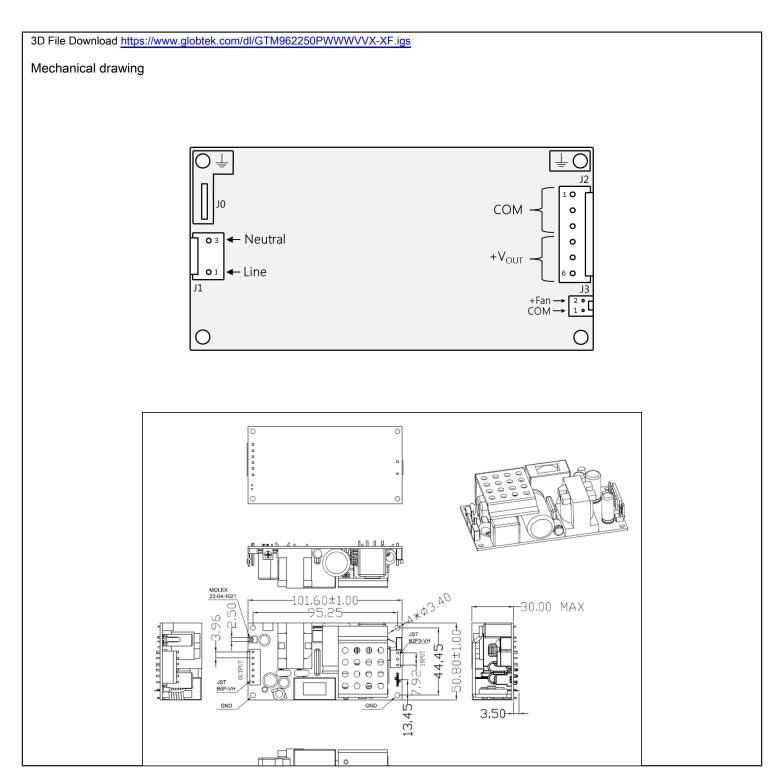
Drawing Title: GTM962250P22516A-F, ICT / ITE / Medical Power Supply, Efficiency Level: USA DOE Level VI / Eco-design Directive 2009/125/EC, (EU) 2019/1782, Case Color/Style: GlobTek Black, Open Frame/ L Frame/Cage/ Potted Internal, Regulated Switchmode AC-DC Power Supply AC Adaptor, Input Rating: 100-240V~, 50-60 Hz, PCB Pins, , Output Rating: 225.00W, 16.0V@14.06A, Pin Out: Pins 1, 2, 3: DC COM Pins 4, 5, 6: +V, Approvals:
