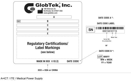
B=P/N: (料号) GTM962250P22515A-F C=Model (型号) GTM962250P22515A-F D=Input (输入)100-240V~, 50-60 Hz, 3A E=Output (输出)15.0 V === 15.0 A, 225.00 W
