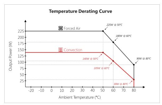
Drawing Title: GTM962250P22512A-F\_, ICT / ITE / Medical Power Supply, Efficiency Level: USA DOE Level VI / Eco-design Directive 2009/125/EC, (EU) 2019/1782, Case Color/Style: GlobTek Black, Open Frame/L Frame/Cage/ Potted Internal, Regulated Switchmode AC-DC Power Supply AC Adaptor, Input Rating: 100-240V~, 50-60 Hz, PCB Pins, , Output Rating: 225.00W, 12.0V@17.55A, Pin Out: Pins 1, 2, 3: DC COM Pins 4, 5, 6: +V, Approvals:
