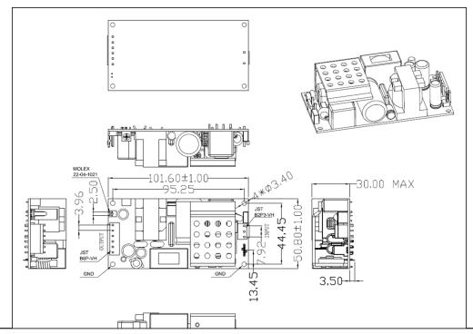
Drawing Title: GTM962250P22512A-F\_, ICT / ITE / Medical Power Supply, Efficiency Level: USA DOE Level VI / Eco-design Directive 2009/125/EC, (EU) 2019/1782, Case Color/Style: GlobTek Black, Open Frame/ L Frame/Cage/ Potted Internal, Regulated Switchmode AC-DC Power Supply AC Adaptor, Input Rating: 100-240V~, 50-60 Hz, PCB Pins, , Output Rating: 225.00W, 12.0V@17.55A, Pin Out: Pins 1, 2, 3: DC COM Pins 4, 5, 6: +V, Approvals:
