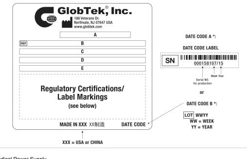
A=Medical Power Supply B=P/N: (料号) GTM41080-1815-FRV C=Model (型号) GTM41080-1817.9-2.9-F(Class I) D=Input (输入)100-240V~, 50-60 Hz, 0.6A E=Output (输出)15.0 V == 1.2 A, 18.00W
