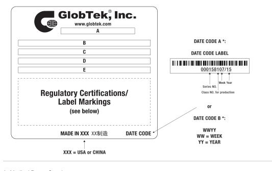
A=Medical Power Supply B=P/N: (料号) GTM41080-1805-FRV C=Model (型号) GTM41080-1807-2.0 D=Input (输入)100-240V~, 50-60 Hz, 0.6A E=Output (输出)5.0 V == 3.6 A, 18.00W
