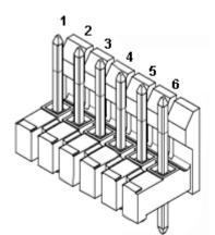
NOTE: pin numbers on output connector do not match naming convention from Molex, they are reversed. Beware of this when specifying and wiring th
