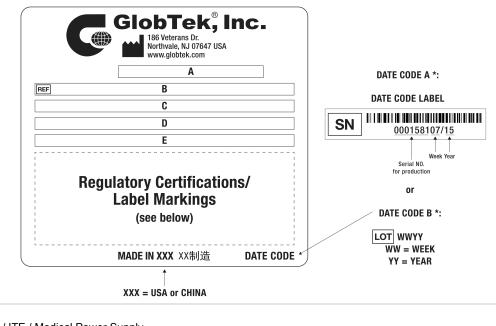
A=ICT / ITE / Medical Power Supply B=P/N: (料号) GTM410602512FWIM(RE) C=Model (型号) GTM41060-2512-FW D=Input (输入)100-240V~, 50-60 Hz, 0.6 A E=Output (输出)12.0 V == 2.08 A, 25.00W
