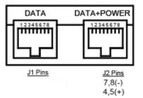
PoE injector wiring Data, Data+Power, RJ45 x 2
