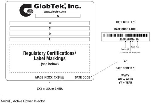
A=POE, Active Power Injector B=P/N: (料号) GT96180-1856T3-APOE C=Model (型号) GT-96180-1856-T3-AP D=Input (输入)100-240V~, 50-60 Hz, 0.6A E=Output (输出)56.0 V === 0.32 A, 18.00W
