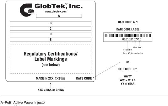
B=P/N: (料号) GT-96300-3656-R3A-AP C=Model (型号) GT-96300-3656-R3A-AP D=Input (输入)100-240V~, 50-60 Hz, 1.0A E=Output (输出)56.0 V === 0.64 A, 36.00W
