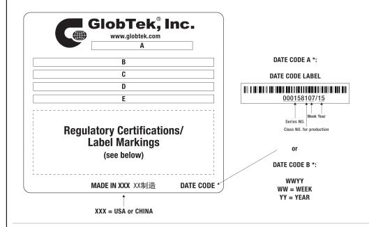
A=PoE, Passive Power Injector B=P/N: (料号) GT-96180-1830-T3-PP C=Model (型号) GT-96180-1830-T3-PP D=Input (输入)100-240V~, 50-60 Hz, 0.6A E=Output (输出)30.0 V === 0.6 A, 18.00W
