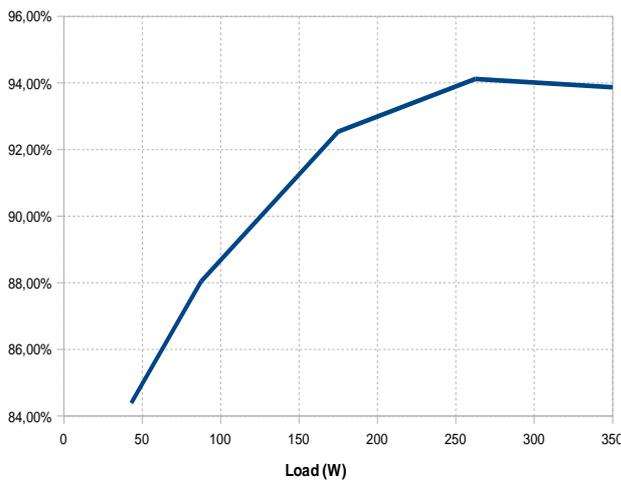
Efficiency versus Load at 230Vac 50Hz
