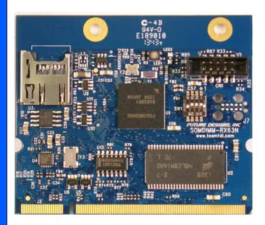
Modular RX63N based Microcontroller Plug-In System-On-Module
