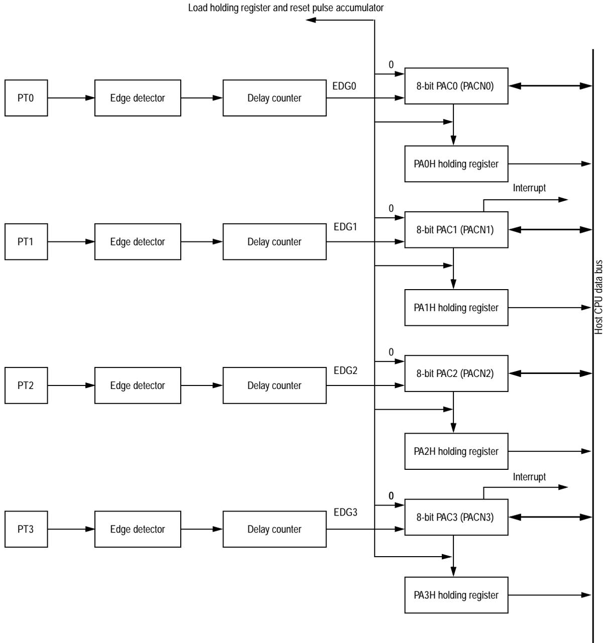
**Figure 15-3. 8-Bit Pulse Accumulators Block Diagram**
