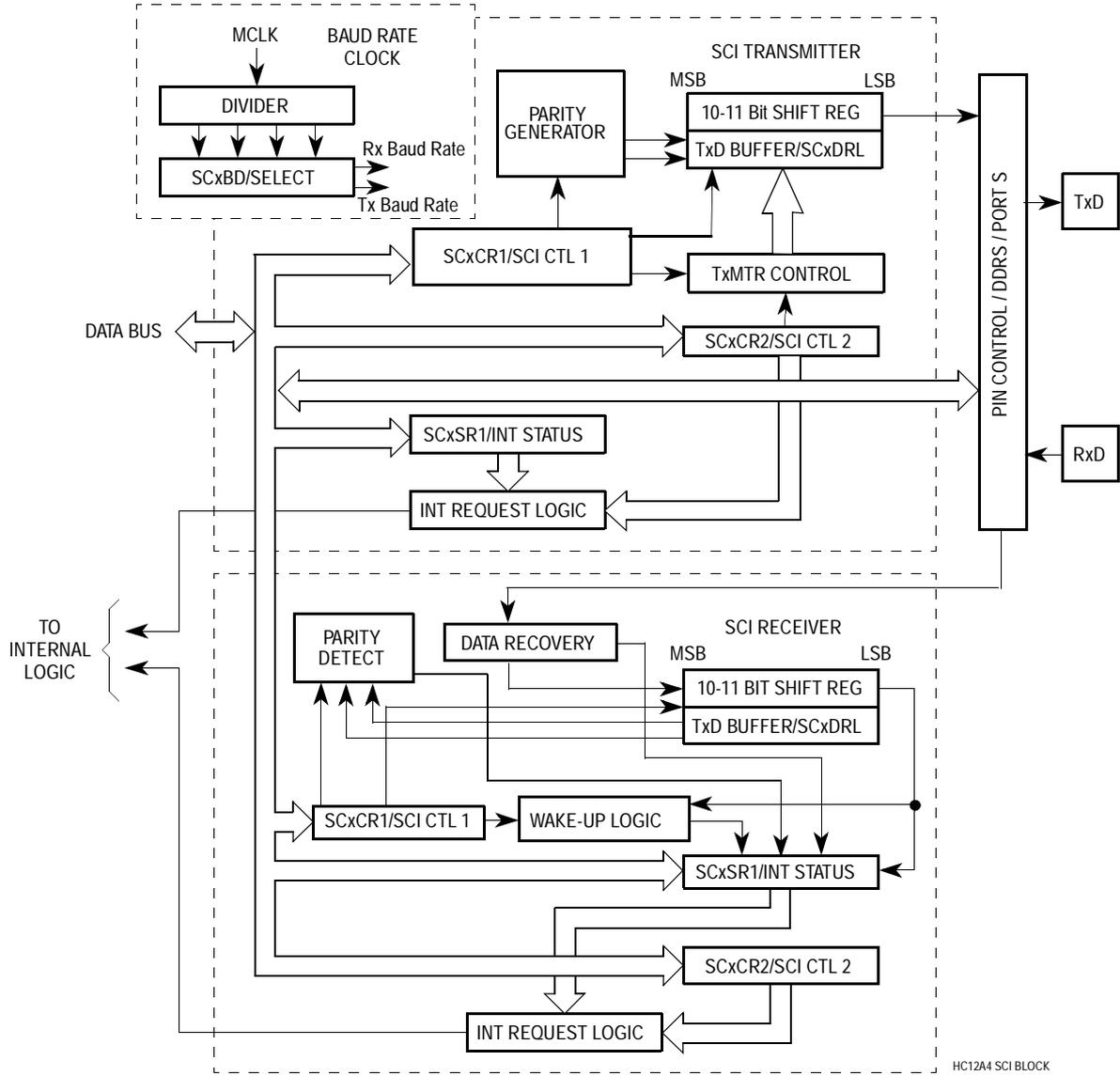
Figure 16-2. Serial Communications Interface Block Diagram
