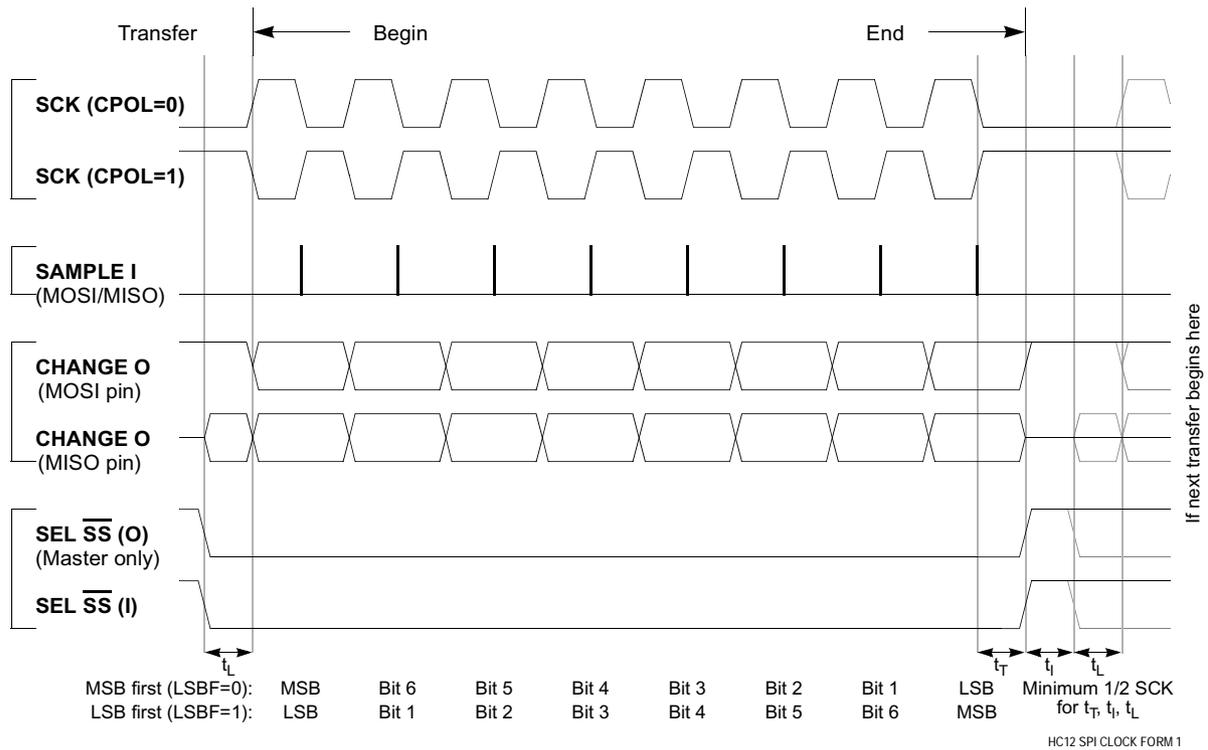
Figure 16-5. SPI Clock Format 1 (CPHA = 1)
