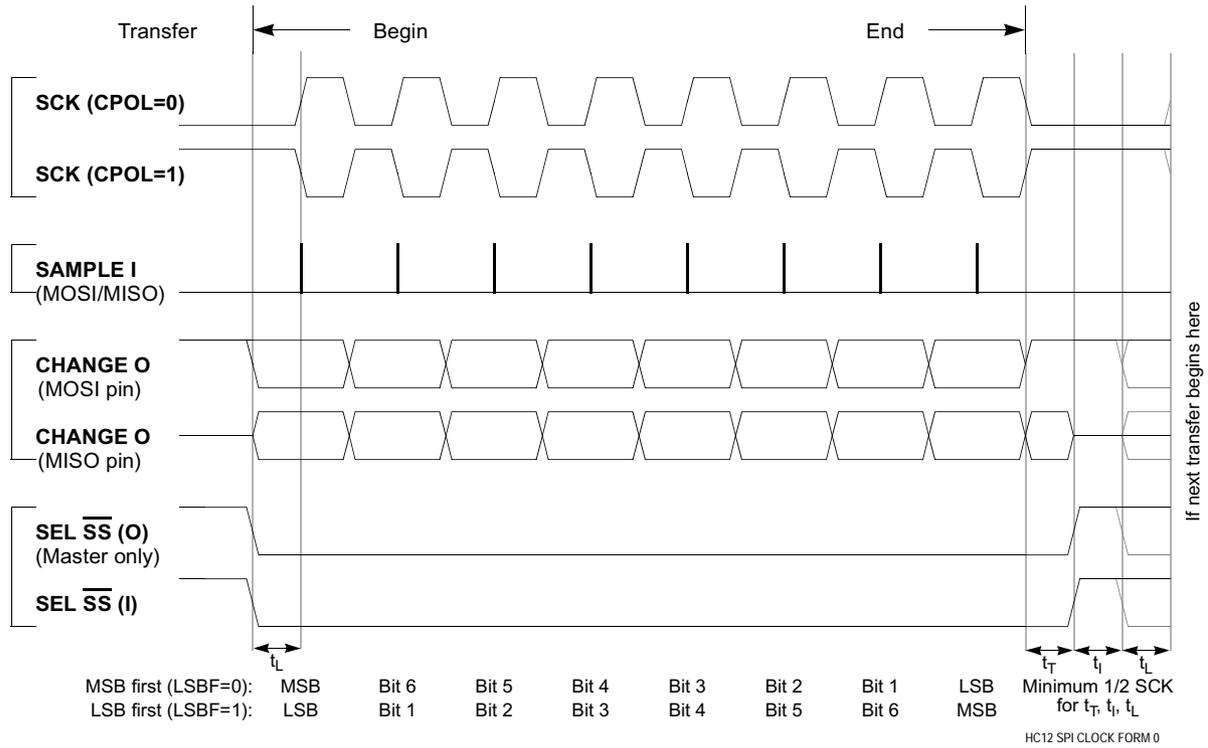
Figure 16-4. SPI Clock Format 0 (CPHA = 0)
