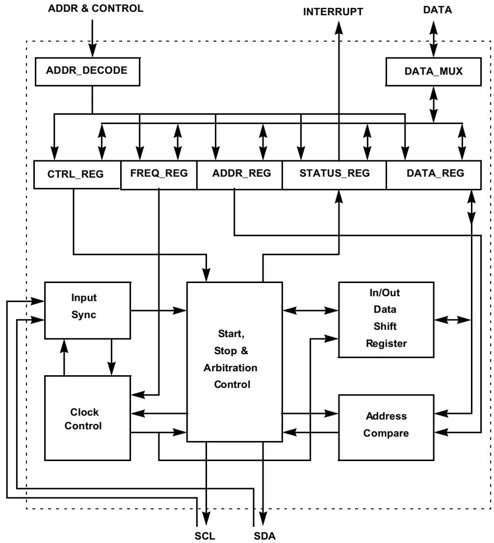
Figure 17-1. IIC Block Diagram
