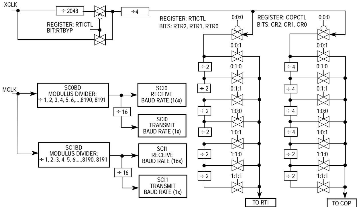
Figure 12-7. Clock Chain for SCI0, SCI1, RTI, COP
