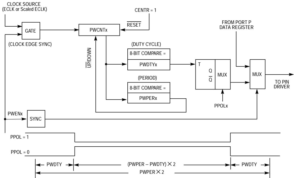
**Figure 14-2. Block Diagram of PWM Center-Aligned Output Channel**
