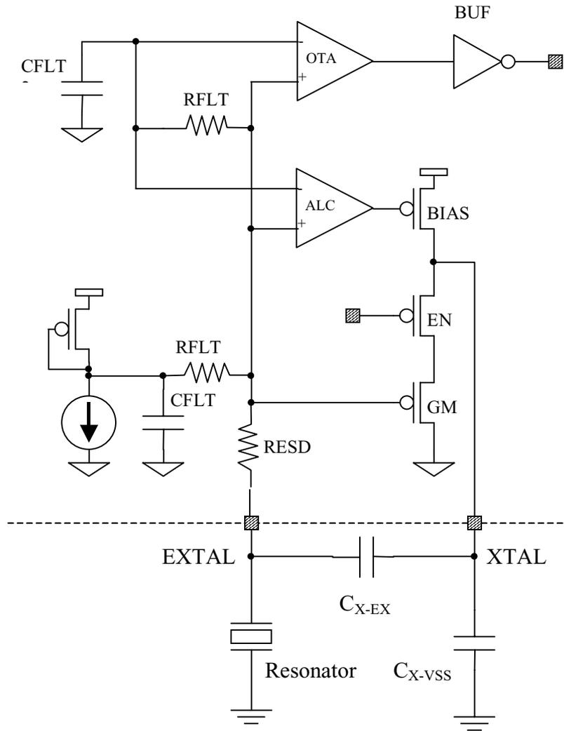
**Figure 13-1. MC68HC912DT128A Colpitts Oscillator Architecture**
