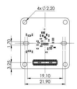
Sensor image optical center is in mechanical board center.
