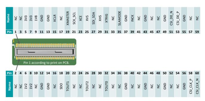
All signals are routed directly from image sensor to connector. Details on specific signals are described in the respective image sensor datasheet.
