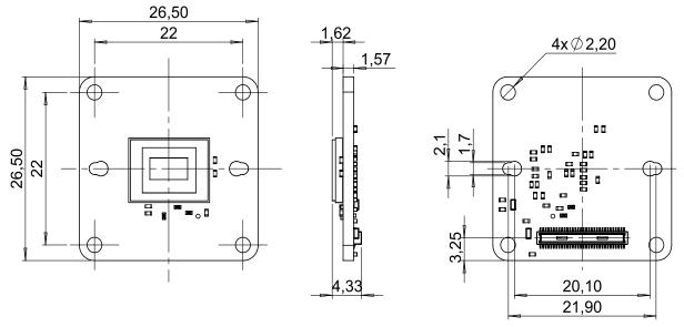
Sensor image optical center is in mechanical board center.
