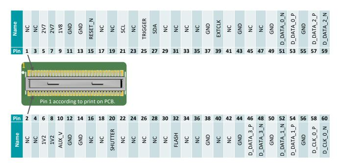
All signals are routed directly from image sensor to connector. Details on specific signals are described in the respective image sensor datasheet.
