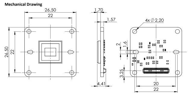
Sensor image optical center is in mechanical board center.
