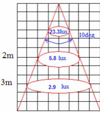
With FHS-HMB1-LL01-z lens: **Medium** beam lens for **Lambertian** Luxeon LED
