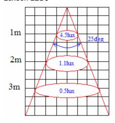
With FHS-HWB1-LB01-z lens: **Wide** beam lens for **Batwing** Luxeon LEDs
