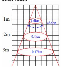
With FHS-HNB1-LL01-z lens: Narrow beam lens for Lambertian Luxeon LED
