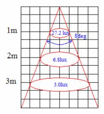
With FHS-HMB1-LB01-z lens: **Medium** beam lens for **Batwing** Luxeon LEDs
