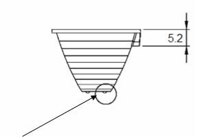
The 4 bumps on the bottom allow the lens to be mounted directly on the Batwing Luxeon LEDs.
