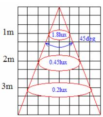
Note: These values have been calculated using the efficiency values of the lens listed above and the formula  ${\bf E}={\bf I}/{\bf d}^2$ , where  ${\bf E}$  is the irradiance in lux,  ${\bf I}$  the intensity in cd, and  ${\bf d}$  the distance between the lens output and the measured point.
