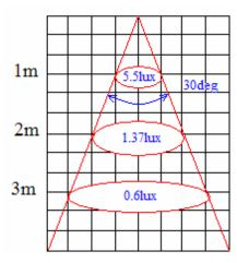
With FHS-HWB1-LL01-z lens: **Wide** beam lens for **Lambertian** Luxeon LED
