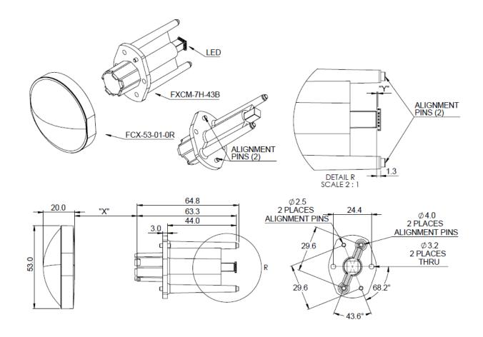
Dimensions are in millimeters.
