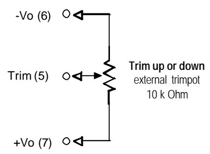
\*) The trim for the dual output is trimming -Vo and +Vo simultaneously and proportional.
