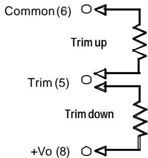
Output may be externally trimmed ( $\pm 10\%$ ) with a fixed resistor or an external trimpot as shown for a single output:
