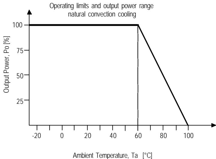
Derating -2.5%/°C at ambient operating temperature range 60°C to 100°C. If ambient temperature ( $T_a$ ) > 60°C then max. allowed output power ( $P_o$ ) can be calculated:
