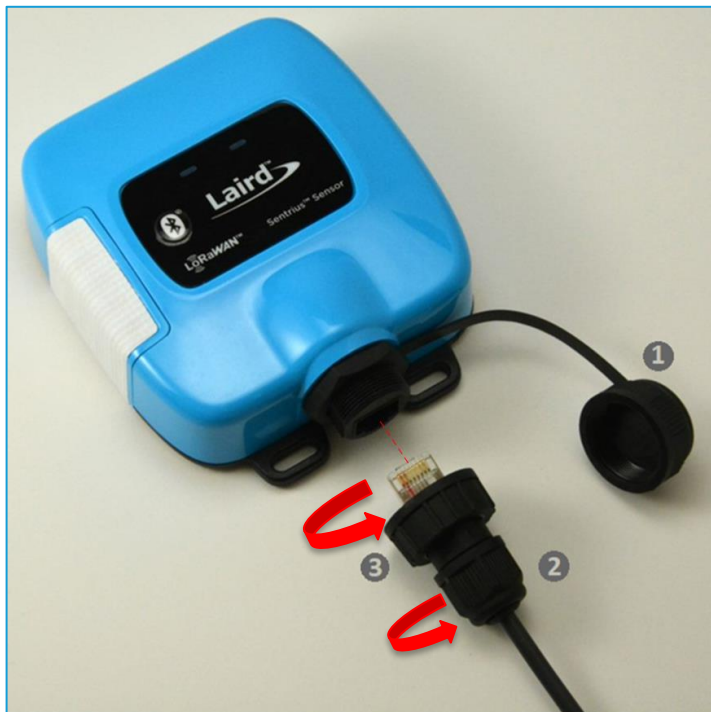
Figure 2: Installing the external temperature sensor
