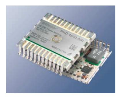
The PKD 4000 SI series of DC/DC power modules are intended to be used as distributed power sources in decentralized 48/60VDC power systems. The PKD series uses a ceramic substrate with thickfilm technology and a high degree of silicon integration. That, together with the electrical design using synchronous rectification gives good thermal management, high reliability and high efficiency.
