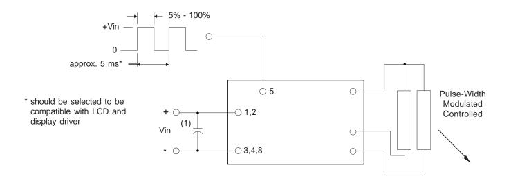
Note 1 Low ESR type input by-pass capacitor (22 uf - 100uf) may be required to reduce reflected ripple.
