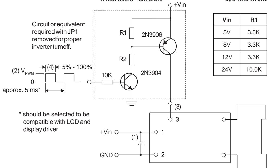
With JP1 in place, a ground applied to the enable pin J1-3 will open the inverter fuse.
