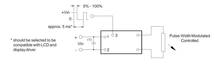
Note 1 Low ESR type Input by-pass capacitor (22 uf - 100uf) may be required to reduce reflected ripple.
