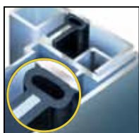
MATERIAL SPECIFICATION • Corner die casting - Aluminum 380 alloy. • Extrusions - Aluminum 6063-T5 alloy.
