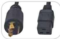
010-9339: NEMA L5-20P to C19 125V, 20A twist-lock 8-foot, 12 AWG/3-wire
