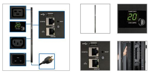
3.7kW vertical PDU distributes and monitors single-phase power in an IT or industrial environment. Built-in Java-free network interface helps you remotely monitor load levels to prevent overloads that cause downtime.
