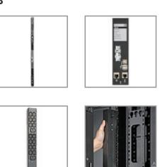
14.5kW 3-phase PDU with multifunction touchscreen LCD distributes and monitors AC power in an IT environment. Built-in Java-free network interface remotely monitors load levels to prevent overloads that cause downtime.
