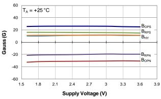
Switch Points vs Supply Voltage
