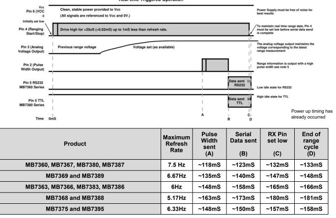
**Pulse Width data sent (Colum A)** - Column A shows the approximate time that the sensor starts to output the pulse width data. The Pulse Width output time can be as short as 300uS (minimum reported distance). For 5 meter sensors, the pulse width can take as long as 5000uS (maximum reported distance) to be sent. For 10 meter sensors the Pulse Width can take as long as 9999uS (maximum reported distance) to be sent.
