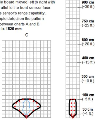
Beam Characteristics are Approximate Beam Pattern drawn to a 1:95 scale for easy comparison to our other products.
